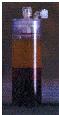
Cylinders are made of Cyrolite Med 2 from Cyro Industries, Rockaway, N.J. Centrifugal force slightly deforms the shape of the cylinder to let the buoy float and let blood cells migrate to the bottom.
