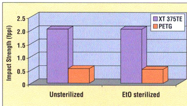
Figure 2. Notched izod impact strength after EtO sterilization.
