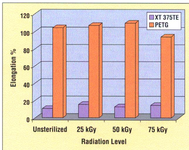
Figure 1. Tensile elongation after E-beam sterilization.
